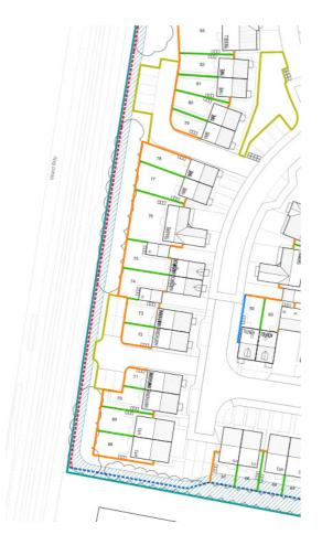
The excerpts shown on this page are taken from the `Enclosures Plan` and show the existing and proposed enclosures at the possible points of vehicle incursion.
